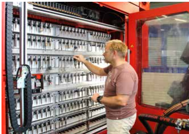
Clear and easy to access: the tool magazine offers space for 186 tools as standard, allowing automatic production
