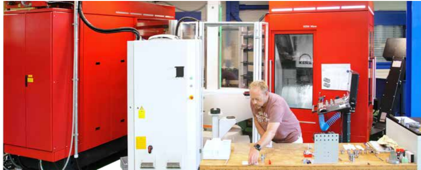
Werner Buschor has placed the two machining centers KERN Micro in such a way that both can be operated by one workpiece changer
